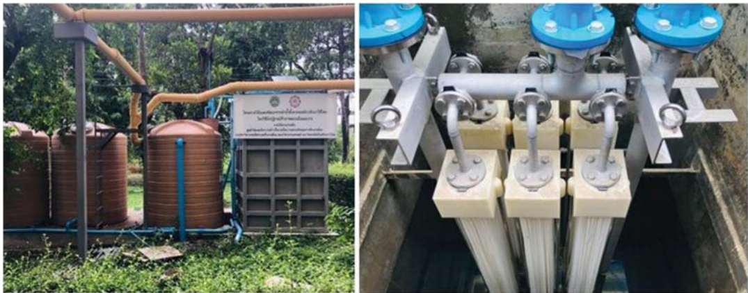
FIGURE 22.7 The MBR pilot plant for greywater treatment at Srinakharinwirot University. Source: From Suthida Theepharakasapan.
